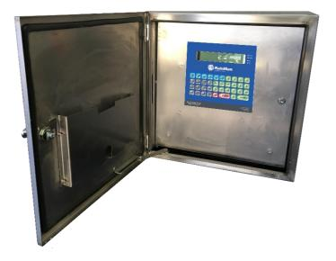
The Type D – 500 x 500 stainless steel enclosure option comes with a key locked door and escutcheon plate. The unit comes prewired with circuit breaker and can be optioned to include prewired lightning protection for input and output wiring.
