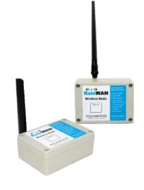
The RainWAN TPL node allows for localised long range, low power wireless networks to provide advanced control over broadacre applications, using the LoRa bandwidth.
