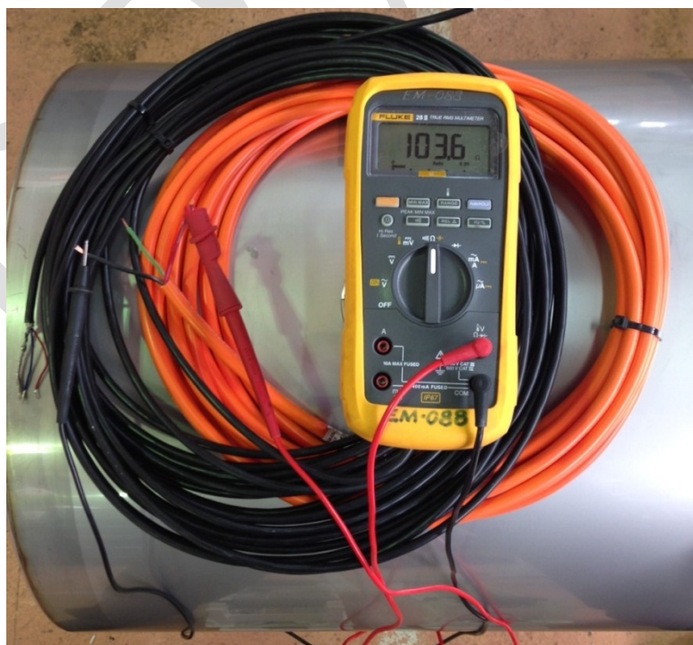
Figure 2: Recording the coil resistance using the RED and BLACK wires of the orange cable.
