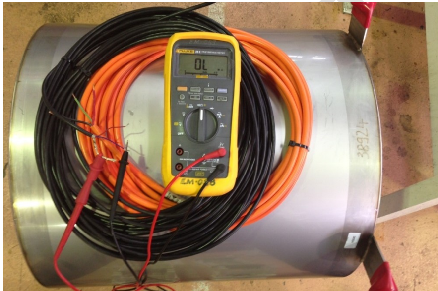
Figure 4: Recording the resistance between BLUE and GREEN wires.
